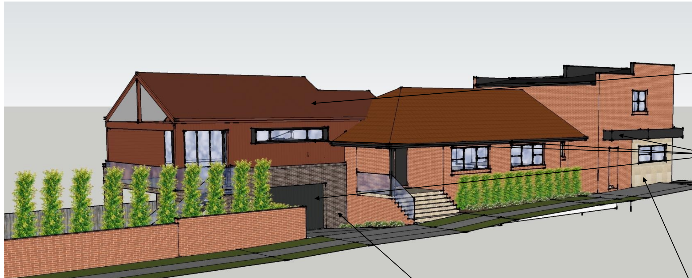
New extension roof, cladding, fascias, gutters, downpipes- Colorbond Copernicus
